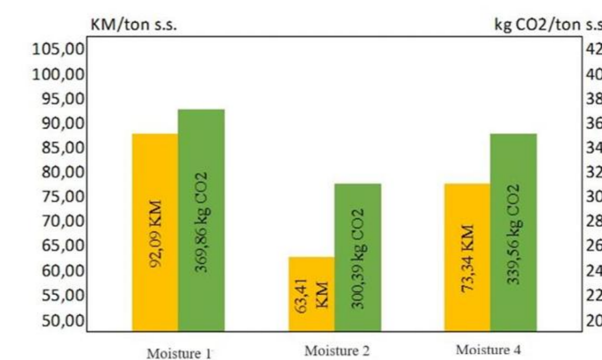
Figure 4. Raw material mixture costs and carbon dioxide emissions per ton of raw material mixture used
